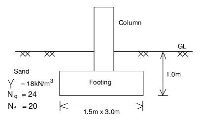
Q.80 The net ultimate bearing capacity (kN/m²) of the footing based on Terzaghi's bearing capacity equation is
