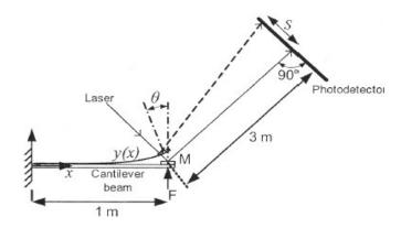
50. The translation S of the spot of laser on the photo-detector when a force of F=1N is applied to the cantilever is:
